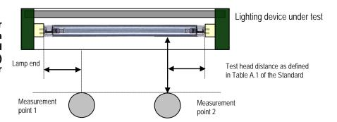
Location of measurement point for lighting equipment with single capped lamp(s) (recessed, surface or pole mounted).
