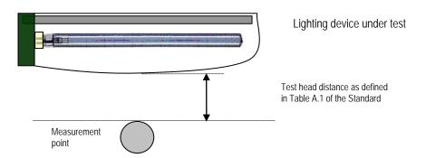
Location of measurement points for lighting equipment with single capped lamp (360° illumination).
